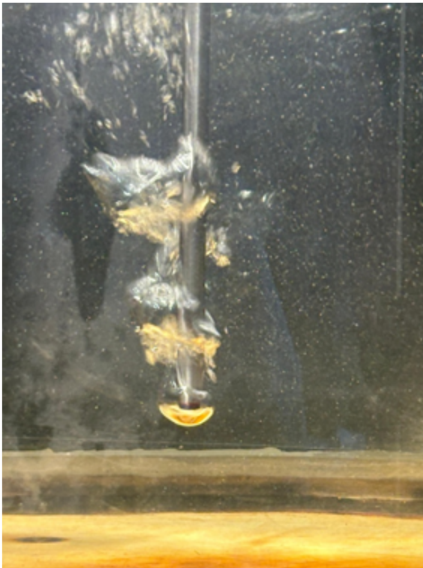
Figure 2. Rising air bubbles coming out of a typical T-shaped lance.
